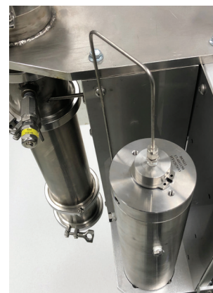
▲ Color Remediation Module
